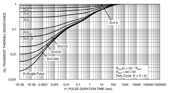
Figure 13. Transient Thermal Resistance
