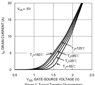
Figure 2. Typical Transfer Characteristic
