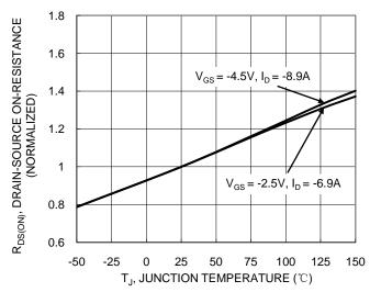
Figure 6. On-Resistance Variation with Junction Temperature
