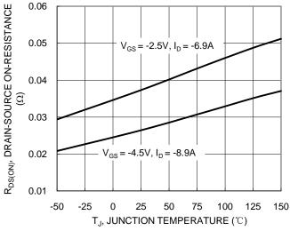
Figure 7. On-Resistance Variation with Junction Temperature
