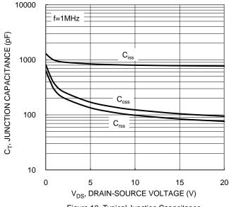
Figure 10. Typical Junction Capacitance
