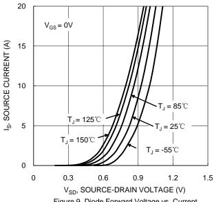
Figure 9. Diode Forward Voltage vs. Current
