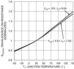
Figure 6. On-Resistance Variation with Junction Temperature
