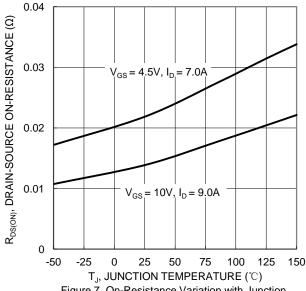
Figure 7. On-Resistance Variation with Junction Temperature
