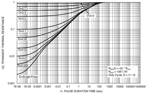
Figure 13. Transient Thermal Resistance
