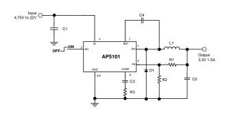
**Figure 1. Typical Application Circuit**
