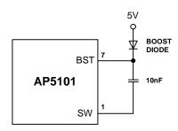
Figure 4. External Bootstrap Diode
