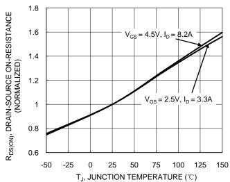
Figure 6. On-Resistance Variation with Junction Temperature
