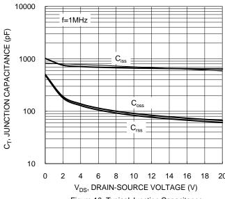
Figure 10. Typical Junction Capacitance
