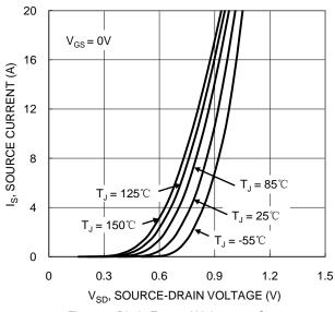
Figure 9. Diode Forward Voltage vs. Current
