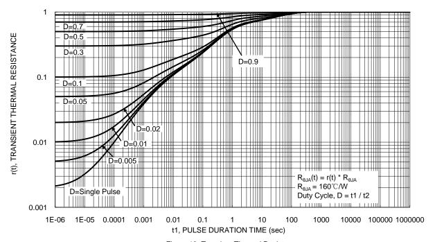
Figure 13. Transient Thermal Resistance
