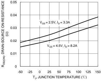
Figure 7. On-Resistance Variation with Junction Temperature
