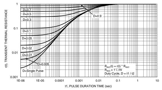
Figure 13. Transient Thermal Resistance
