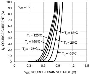
Figure 9. Diode Forward Voltage vs. Current
