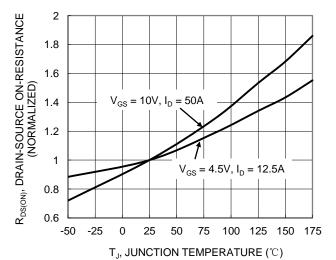
Figure 6. On-Resistance Variation with Junction Temperature
