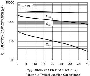
Figure 10. Typical Junction Capacitance
