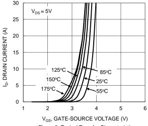
Figure 2. Typical Transfer Characteristic
