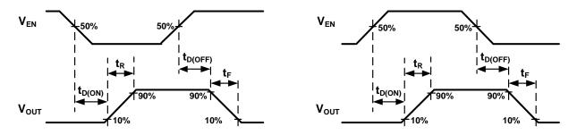
Figure 1. Voltage Waveforms: AP2181D (Left), AP2191D (Right)
