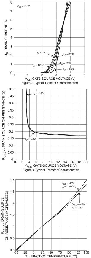
Figure 6 On-Resistance Variation with Temperature
