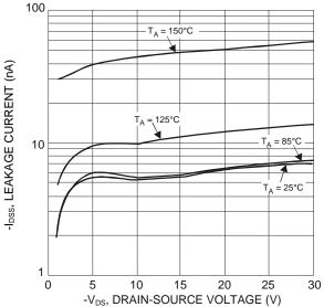
Fig. 9 Typical Drain-Source Leakage Current vs. Voltage
