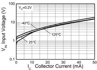
**Input Voltage v Collector Current**
