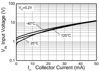
Input Voltage v Collector Current
