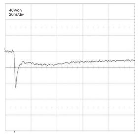
Figure 2 IEC 6100-4-2 Clamping Voltage -8kV Contact
