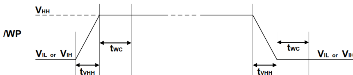
Figure 9-2. ACC Program Acceleration Timing and Voltage Levels
