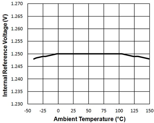
Figure 7.1 : Typical VPS Pin Internal Reference Voltage Threshold (Falling Edge) vs. Temperature
