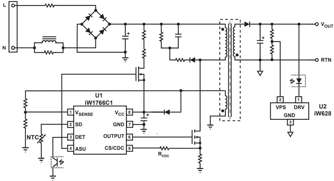
Figure 3.2: iW628 Typical Application Circuit (Using iW1766C1 as Primary-Side Controller)
