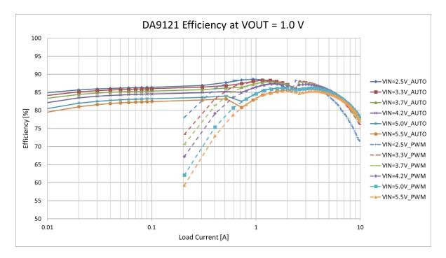
DA9121 operates as a dual-phase buck converter, delivering up to 10 A output current. The output voltage is programmable from 0.3 V to 1.9 V in 10 mV increments. The input voltage range of 2.5 V to 5.5 V makes it suitable for a wide variety of low-voltage systems, including all Li-Ion battery powered applications. To guarantee the highest accuracy and to support multiple PCB routing scenarios without loss of performance, a remote differential sensing capability is implemented.
