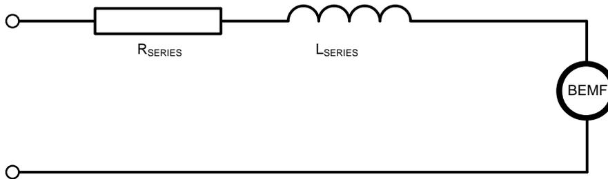
Figure 21: Equivalent Electrical Model of an Actuator
