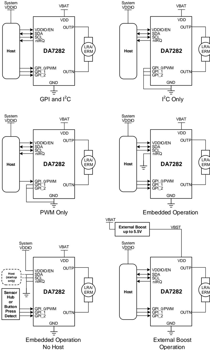
Figure 1: System Diagrams
