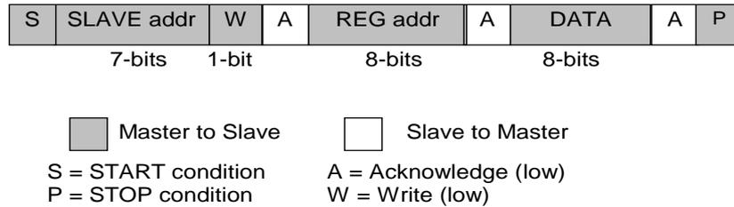
**Figure 35: I<sup>2</sup>C Byte Write (SDA line)**
