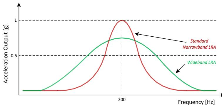
**Figure 6: Narrowband and Wideband LRA Response across Frequency**
