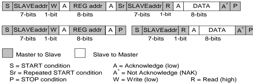
**Figure 36: Examples of the I<sup>2</sup>C Byte Read (SDA line)**
