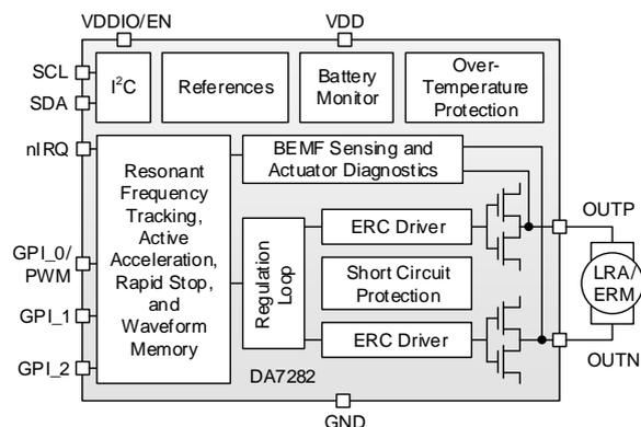
LRA/ERM Ultra-Low Power Haptic Driver with Multiple Input Triggers and Integrated Waveform Memory
