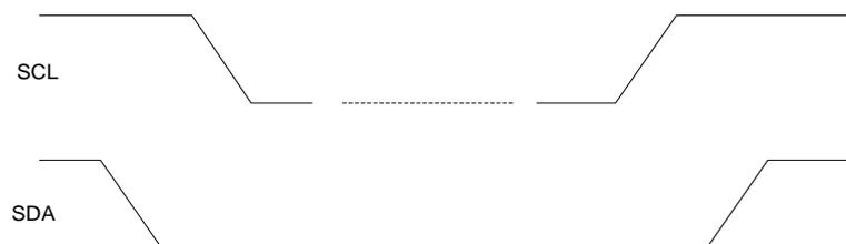
Figure 34: I<sup>2</sup>C START and STOP Conditions
