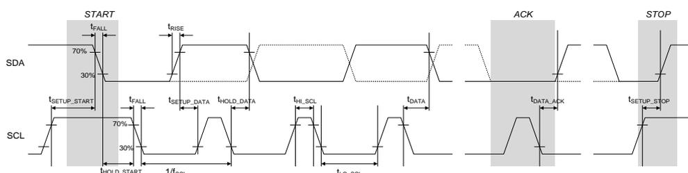
**Figure 4: I<sup>2</sup>C Interface Timing**
