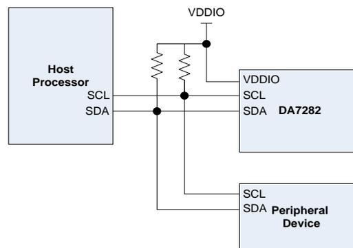
Figure 33: Schematic of the I<sup>2</sup>C Control Interface Bus
