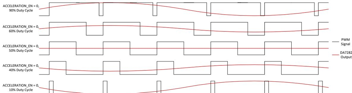
Figure 9: Example PWM Inputs with `ACCELERATION_EN = 0`
