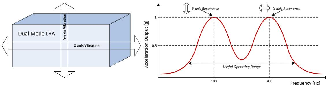
**Figure 7: Dual Mode LRA Response across Frequency**
