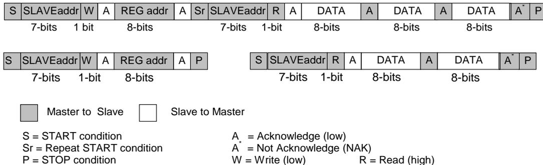
**Figure 37: Examples of I<sup>2</sup>C Page Read (SDA line)**
