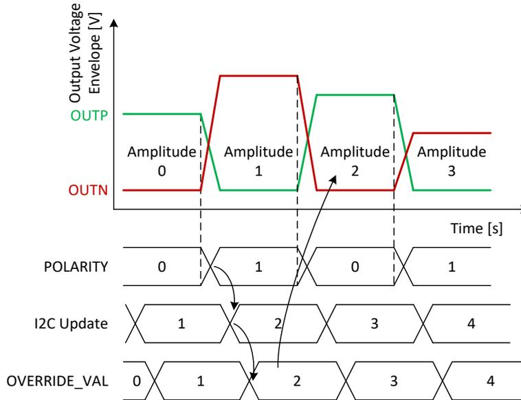
Figure 20: Polarity Timing Relationship
