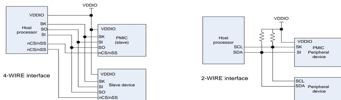
**Figure 19: Schematic of 4-WIRE and 2-WIRE Power Manager Bus**
