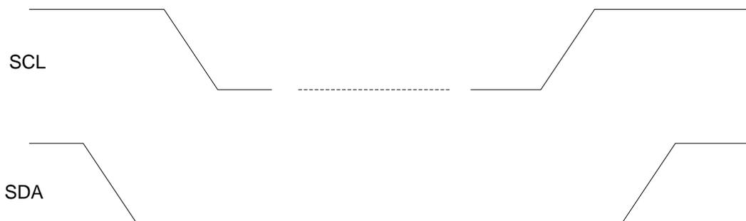
**Figure 24: Timing of 2-WIRE START and STOP Condition**
