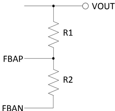
**Figure 17: Resistive Divider from VOUT to FBAN**
