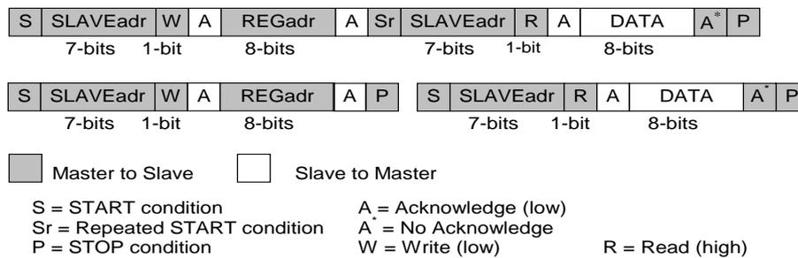
**Figure 26: Examples of 2-WIRE Byte Read (SDA Line)**
