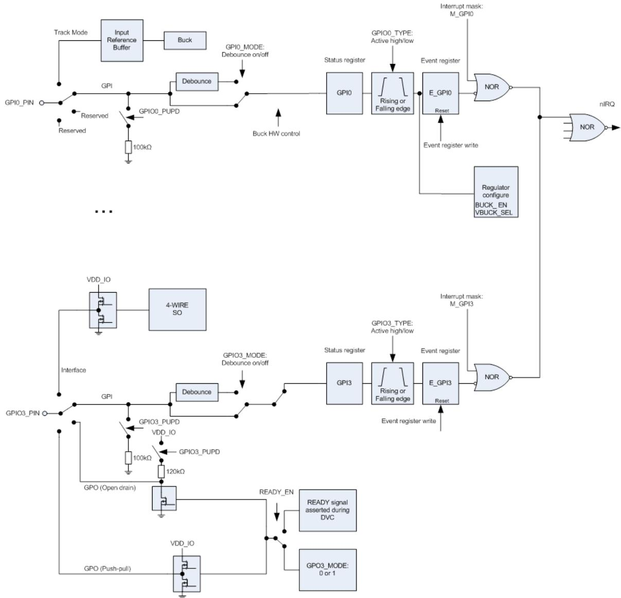
**Figure 18: GPIO Principle of Operation (example paths)**
