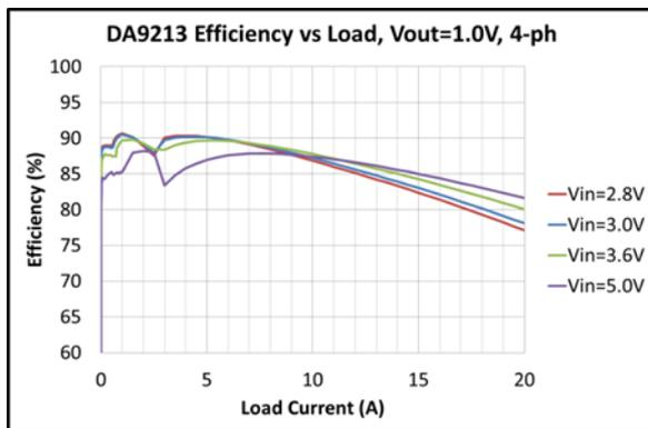
Figure 9: 4 Phase Auto-Mode, 0 to 20 A (Linear)
