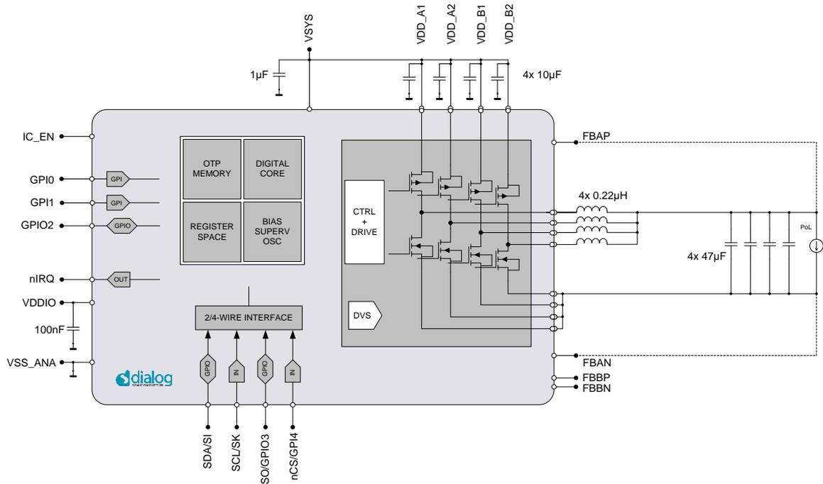
Figure 1: DA9213, DA9214, and DA9215 System Diagram
