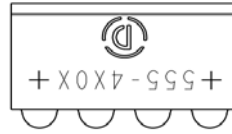
OLD 555-4XXX F HOUSING WITH PRINTED P/N AND POLARITY MARKING
