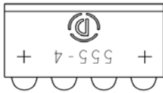
NEW 555-4XXX F WITH ENGRAVED SERIES NUMBER AND POLARITY MARKINGS
