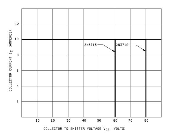
FIGURE 6. Safe operating area for switching between saturation and cutoff (clamped inductive load).
