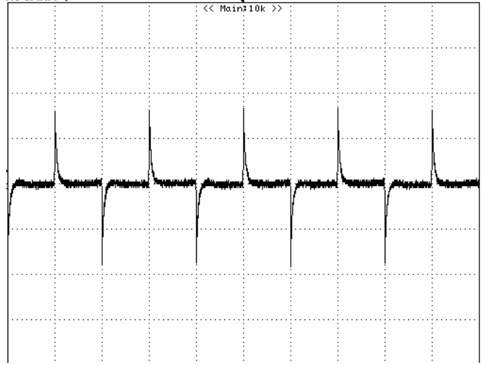
Figure 18: Typical transient response to step load change at 1A/\mu S from 100%~ 0%~100% of I_o , max at 12Vin, 2.5Vout ( C_{out} = 1\mu F ceramic, 47\mu F+10\mu F ceramic) CH1 : VOUT, 0.1V/div, 5mS/div
