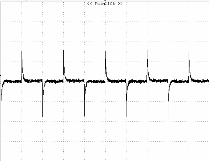
Figure 17: Typical transient response to step load change at 1A/\mu S from 100%~ 0%~100% of I_o , max at 12Vin, 5.0Vout ( C_{out} = 1\mu F ceramic, 47\mu F+10\mu F ceramic) CH1 : VOUT, 0.1V/div, 5mS/div
