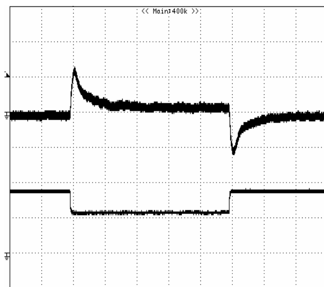
Figure 9: Output voltage response to step-change in load current (75%-50%-75% of I_o , max; di/dt = 2.5A/\mu s ). Load cap: 330\mu F , 35m\Omega ESR solid electrolytic capacitor and 1\mu F ceramic capacitor. Top Trace: V_{out} (100mV/div, 200us/div), Bottom Trace: I_{out} (5A/div). Scope measurement should be made using a BNC cable (length shorter than 20 inches). Position the load between 51 mm to 76 mm (2 inches to 3 inches) from the module
