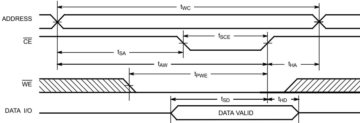
Figure 11. Write Cycle No. 3 ( $\overline{WE}$  Controlled,  $\overline{OE}$  LOW) [27, 30]
