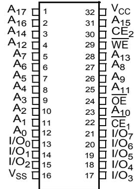
Figure 4. 32-pin STSOP (Top View)
