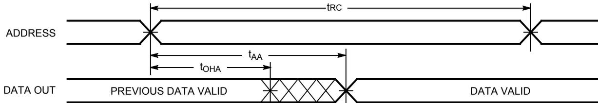
Figure 8. Read Cycle No. 2 ( $\overline{\text{OE}}$  Controlled) [20, 21, 22]
