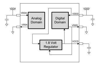
There are two distinct modes of operation. In Mode 1, the supply voltage range is 1.8 V to 5.5 V (unregulated externally; internal regulator operational). In Mode 2, the supply range is  $1.8 \text{ V} \pm 5\%$  (externally regulated; 1.71 to 1.89, internal regulator bypassed).
