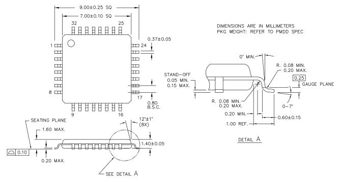
Figure 10. 32-pin TQFP (7 × 7 × 1.4 mm) Package Outline, 51-85088
