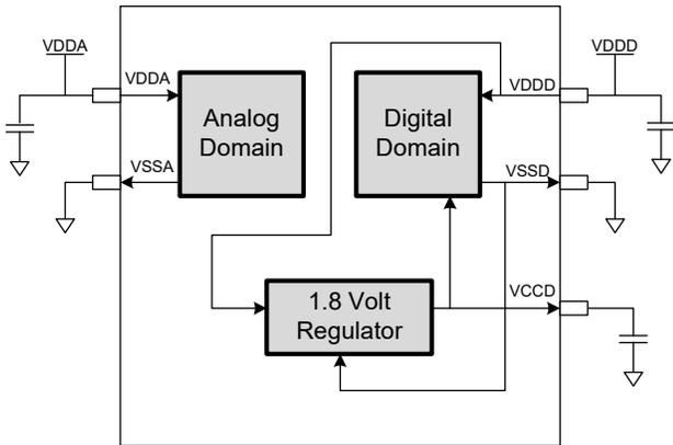
There are two distinct modes of operation. In Mode 1, the supply voltage range is 1.8 V to 5.5 V (unregulated externally; internal regulator operational). In Mode 2, the supply range is 1.8 V ±5% (externally regulated; 1.71 to 1.89, internal regulator bypassed).
