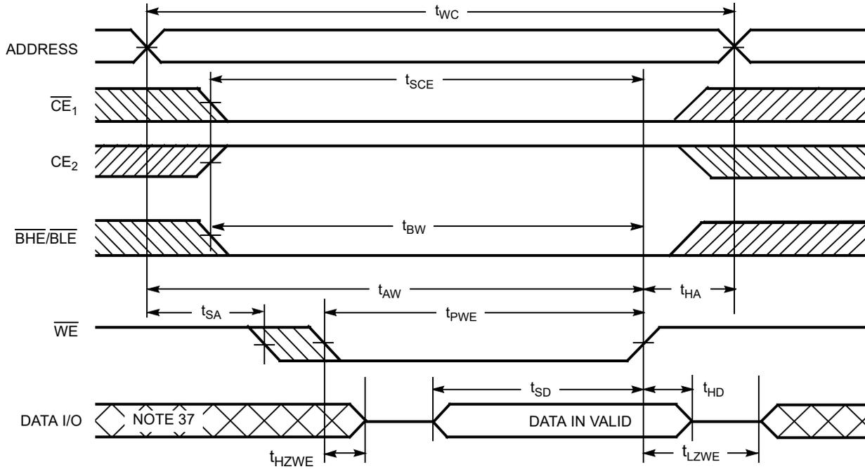
Figure 10. Write Cycle No. 4 ( $\overline{BHE}/\overline{BLE}$  controlled,  $\overline{OE}$  LOW)<sup>[36]</sup>
