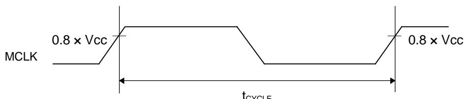
**External bus signal input/output characteristics**
