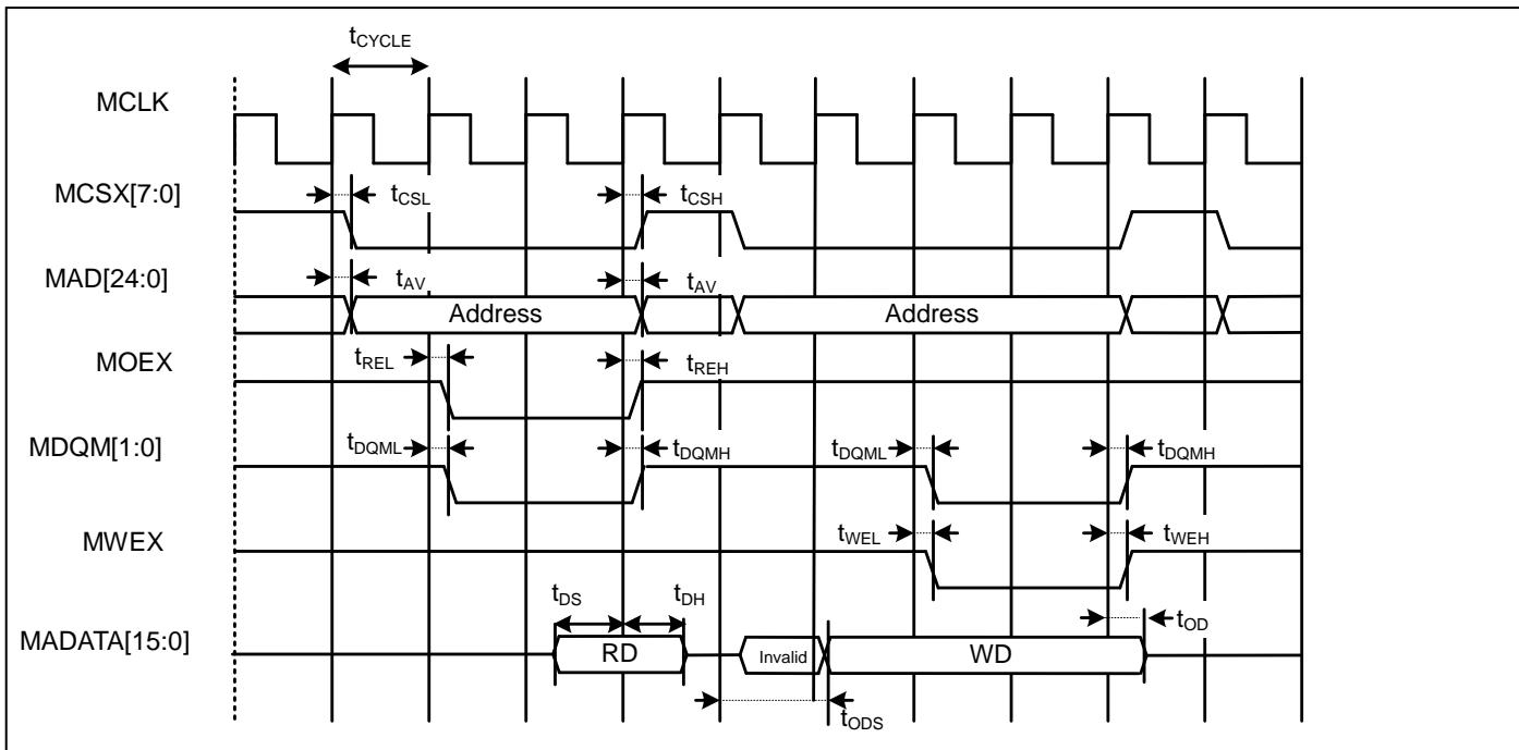
**Multiplexed Bus Access Asynchronous SRAM Mode**
