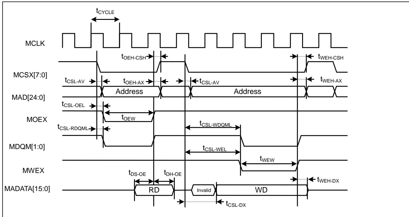
**Separate Bus Access Synchronous SRAM Mode**
