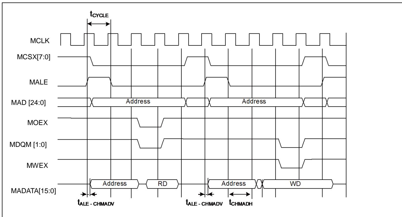
**Multiplexed Bus Access Synchronous SRAM Mode**
