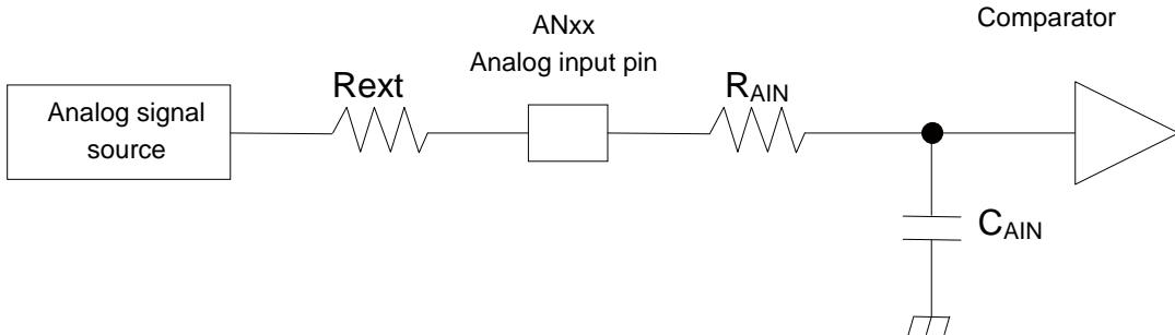
(Equation 1)  $T_s \geq (R_{AIN} + R_{ext}) \times C_{AIN} \times 9$
