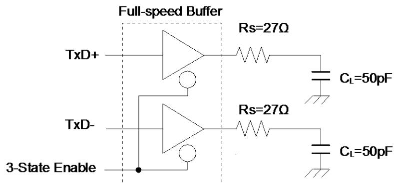
\*6: USB Full-speed connection is performed via twist pair cable shield with  $90\Omega \pm 15\%$  characteristic impedance (Differential Mode). USB standard defines that output impedance of USB driver must be in range from  $28\Omega$  to  $44\Omega$ . So, discrete series resistor ( $Rs$ ) addition is defined in order to satisfy the above definition and keep balance.
