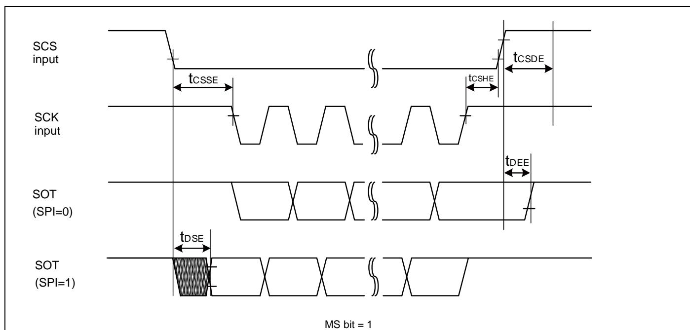
**When using high-speed synchronous serial chip select (SCINV = 1, CSLVL=1)**
