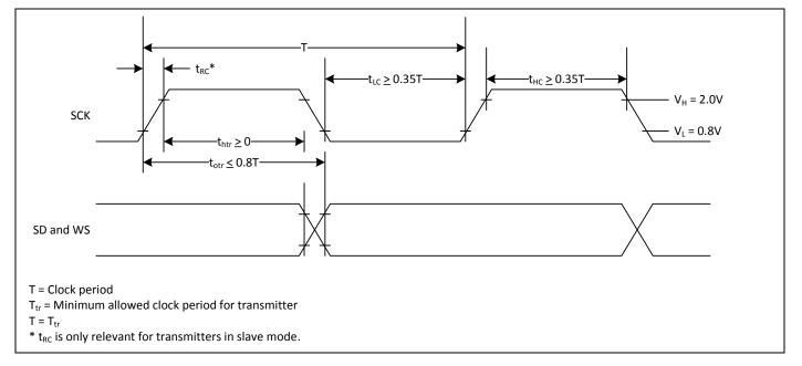
Figure 17. I<sup>2</sup>S Transmitter Timing
