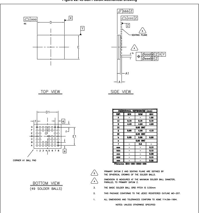
Figure 22. 49-Ball FcBGA Mechanical Drawing
