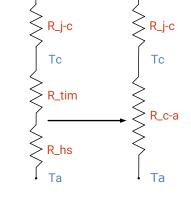
As the figure at right shows, the R\_c-a value is the sum of the thermal resistance of the TIM (R\_tim) plus the thermal resistance of the heat sink (R\_hs).
