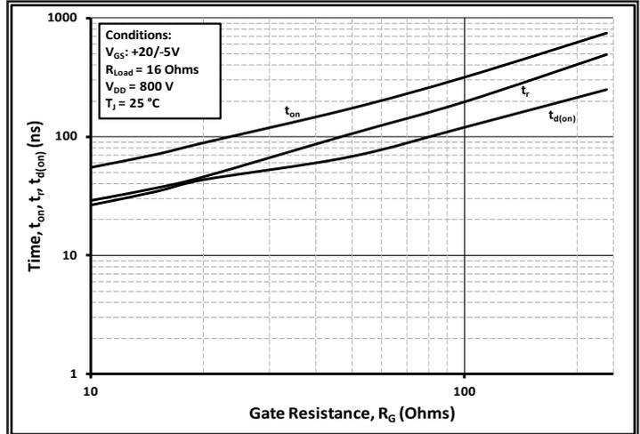
Figure 22. Turn-on Timing vs. External Gate Resistor
