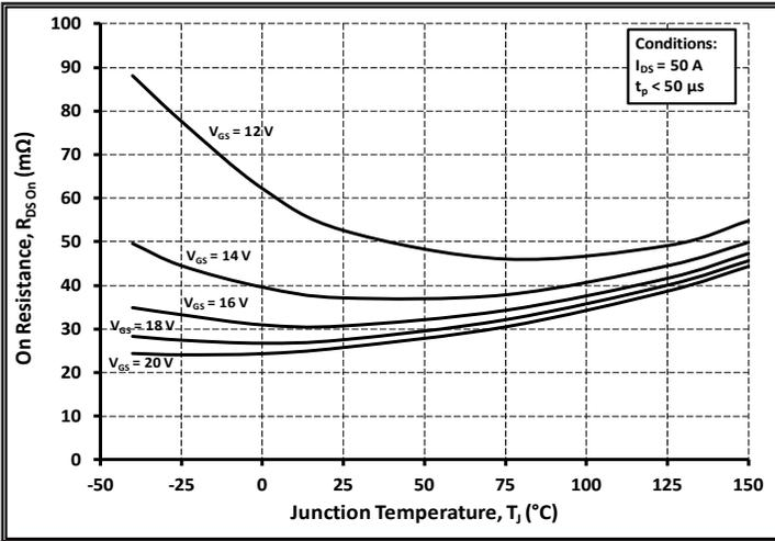
Figure 7. On-Resistance vs. Temperature for Various Gate-Source Voltages
