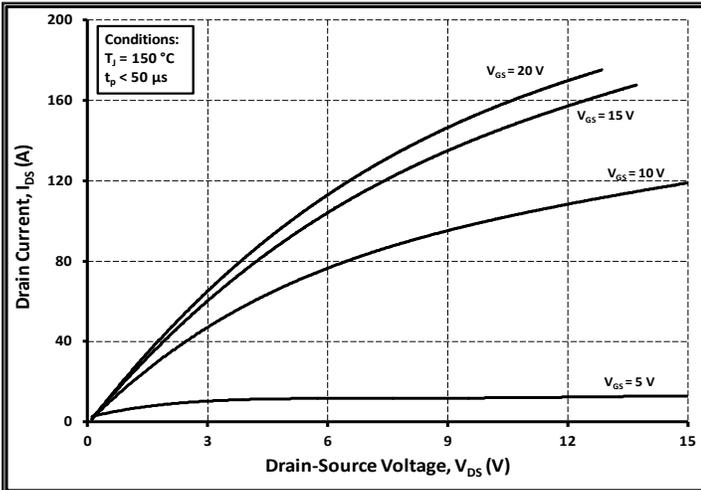
Figure 3. Typical Output Characteristics  $T_j = 150\text{ }^\circ\text{C}$
