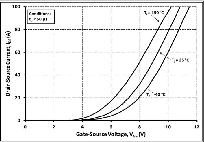
Figure 8. Transfer Characteristic for Various Junction Temperatures
