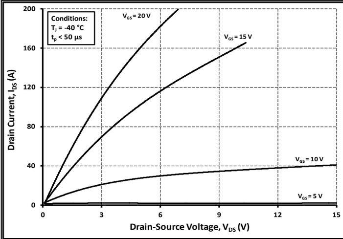
Figure 1. Typical Output Characteristics  $T_j = -40\text{ }^\circ\text{C}$
