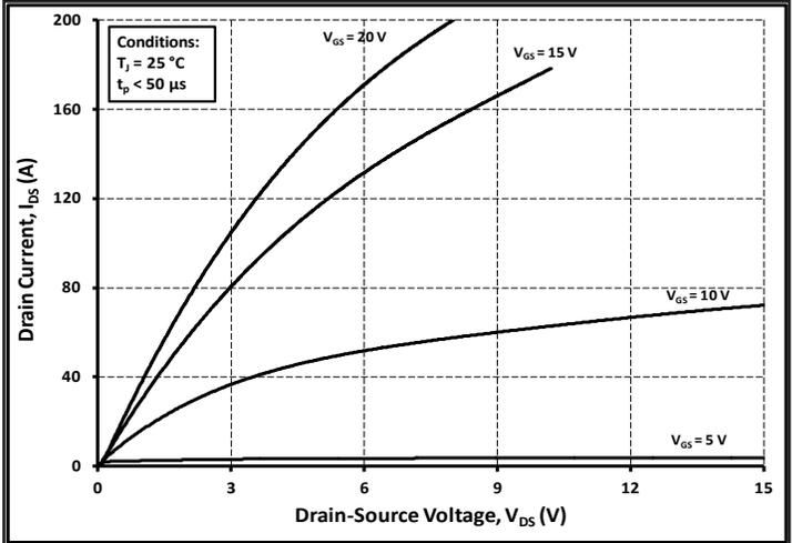
Figure 2. Typical Output Characteristics  $T_j = 25\text{ }^\circ\text{C}$
