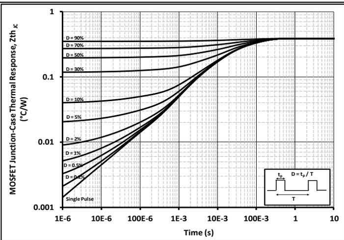
Figure 29. MOSFET Junction to Case Thermal Impedance
