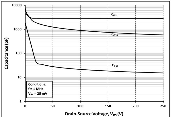
Figure 16. Typical Capacitances vs. Drain-Source Voltage (0 - 250 V)
