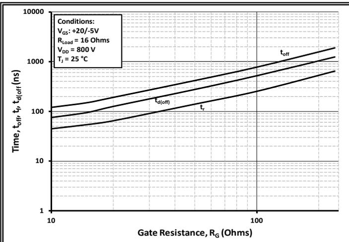
Figure 23. Turn-off Timing vs. External Gate Resistor
