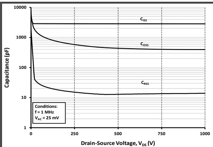
Figure 17. Typical Capacitances vs. Drain-Source Voltage (0 - 1 kV)
