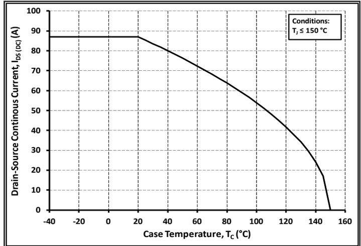
Figure 26. Continuous Drain Current Derating vs Case Temperature
