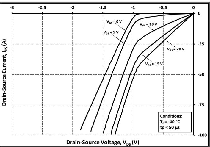
Figure 12. 3<sup>rd</sup> Quadrant Characteristic at -40 °C
