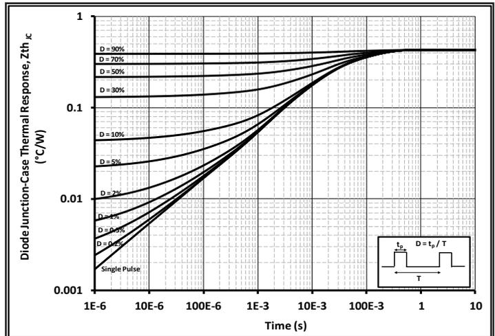
Figure 30. Diode Junction to Case Thermal Impedance
