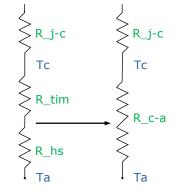
As the figure at right shows, the  $R_c$ -a value is the sum of the thermal resistance of the TIM ( $R_t$ ) plus the thermal resistance of the heat sink ( $R_h$ ).
