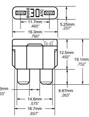
Catalog Symbol: ATC Fast-Acting Ampere Rating: 1 to 40 Amperes Voltage Rating: 32 Volts DC (or less) Interrupting Rating: 1,000 Amperes Agency Approvals: U.L. Recognized, (3-40A) Guide JFHR2, File E56412
