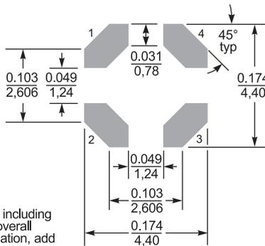
\* Dimensions are of the case not including the termination. For maximum overall dimensions including the termination, add 0.005 in / 0.13 mm.
