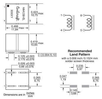
**Packaging** 400/13" reel Plastic tape: 24 mm wide, 0.5 mm thick, 16 mm pocket spacing, 10.8 mm pocket depth
