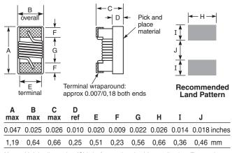
**Note:** Height dimension (C) is before optional solder application. For maximum height dimension including solder, add 0.006 in / 0,152 mm.
