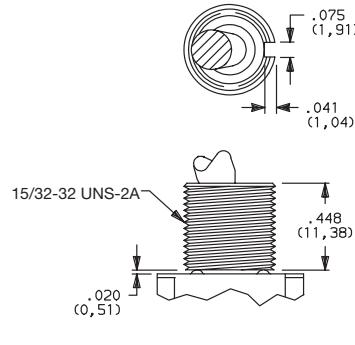
Will withstand 12 in./lbs. of torque with no distortion.
