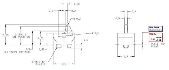
Note: C&K Drawing General Sheet Tolerance for this switch & custom number options will be changed from: +/-0.3mm to +/-0.2mm
