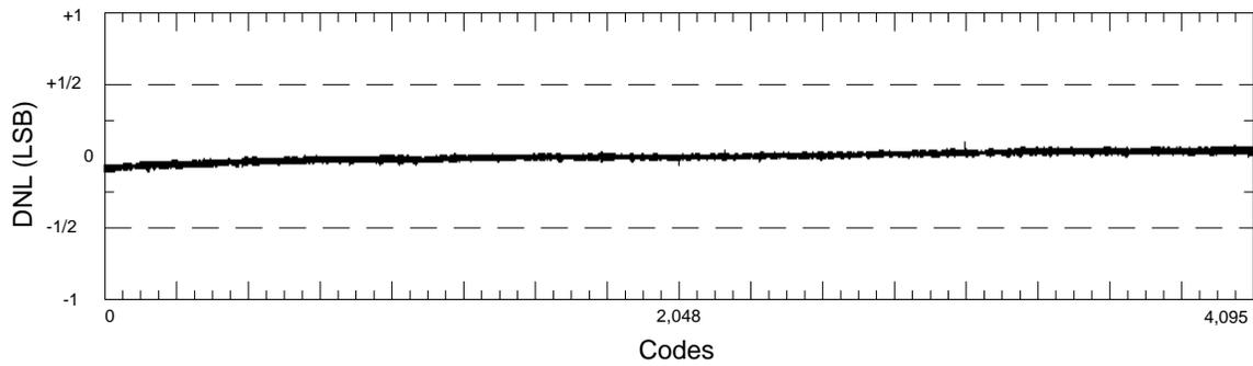
**Figure 15. CS5012 Differential Nonlinearity Plot**
