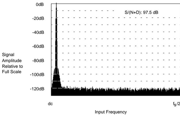
**Figure 23. Plot of Ideal 16-bit ADC**
