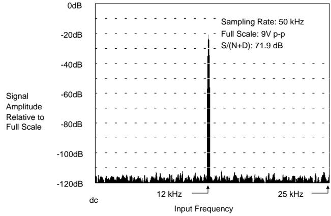
**Figure 34. CS5016 FFT plot with 12 kHz -20 dB Input**
