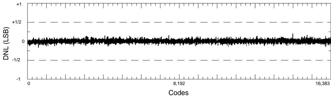
**Figure 16. CS5014 Differential Nonlinearity Plot**
