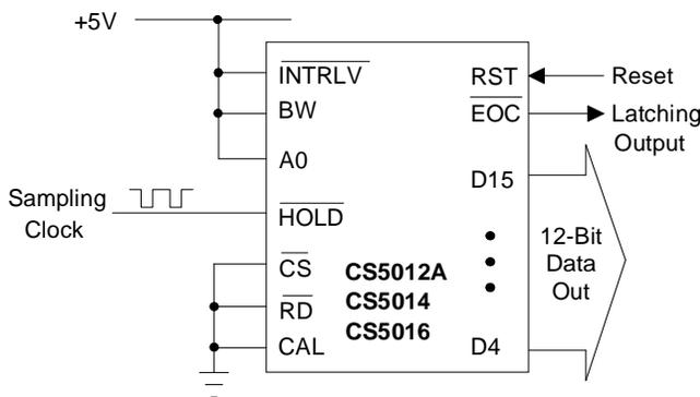
**Figure 8. Microprocessor-Independent Connections**
