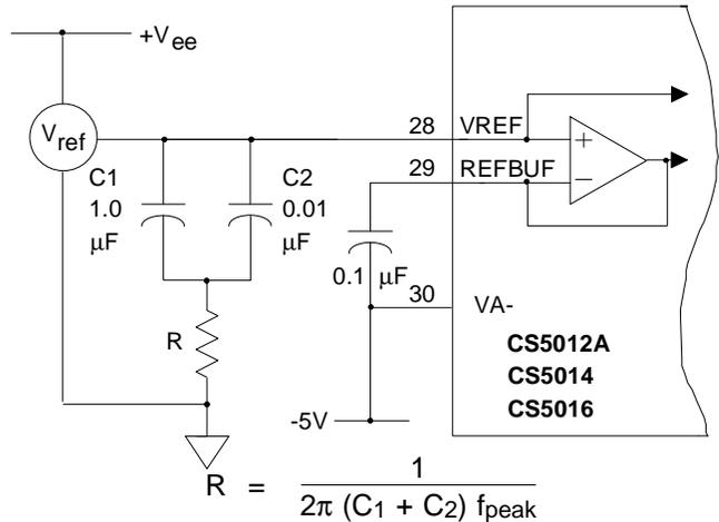
**Figure 10. Reference Connections**
