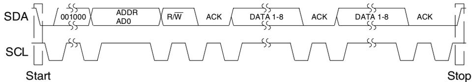
**Figure 12. Control Port Timing, I<sup>2</sup>C mode**
