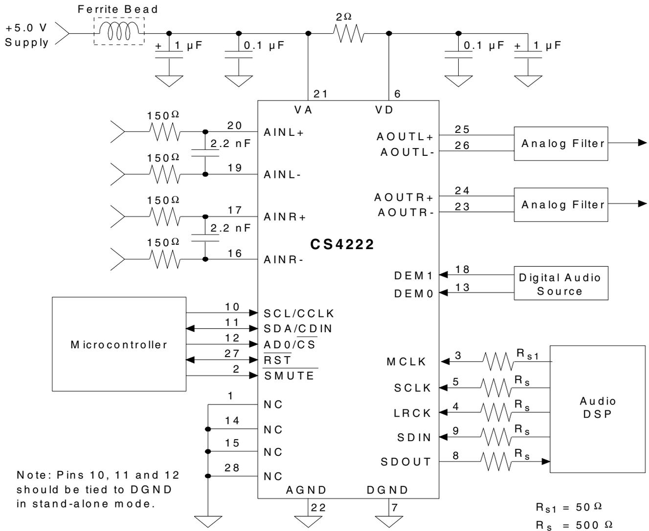
Figure 4. CS4222 Recommended Connection Diagram
