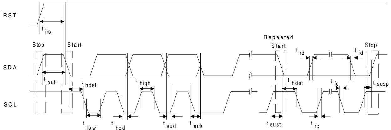
**Figure 3. Control Port Timing - I<sup>2</sup>C Mode**
