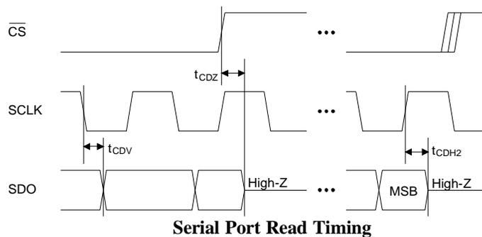
13. Serial port write must precede a port read to provide address information.
