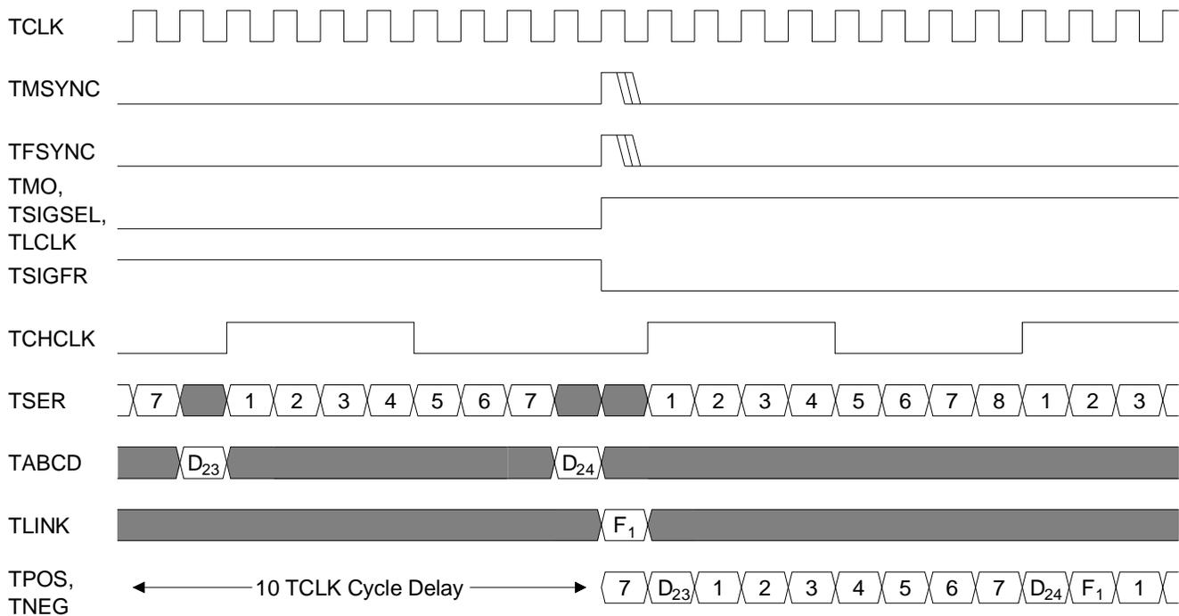
**Figure 5. Bit Level Transmit Timing (193E, signaling enabled)**
