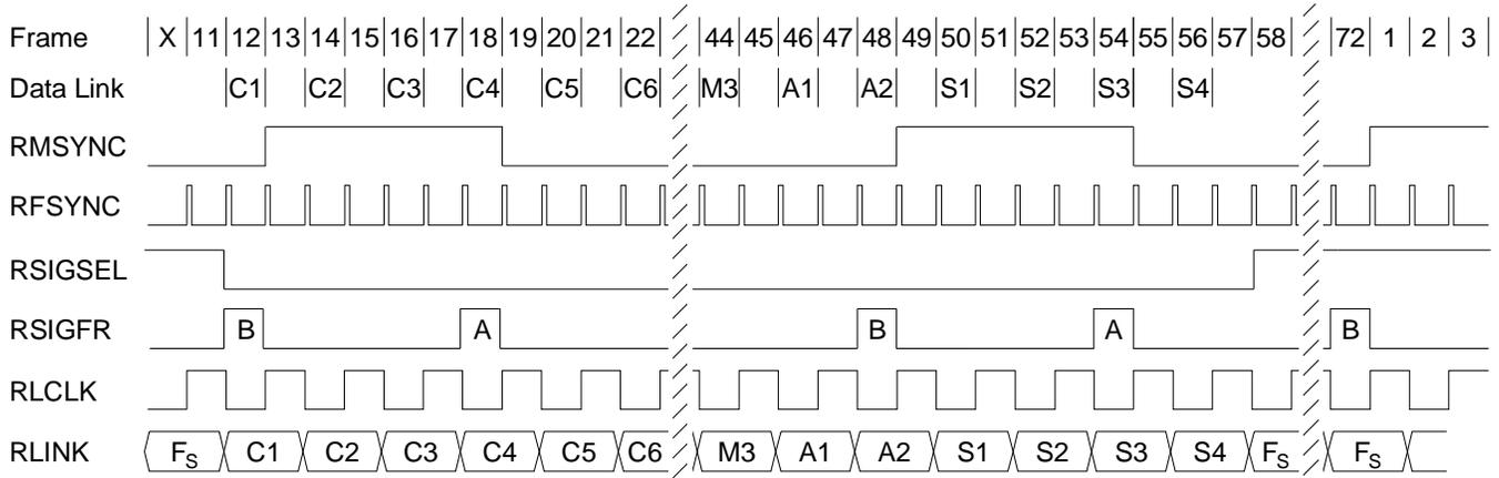
**Figure 17. SLC-96<sup>®</sup> Multiframe Receive Timing**
