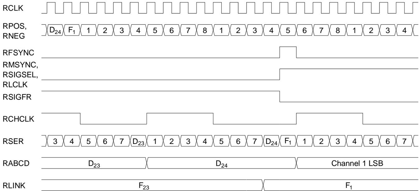
**Figure 14. Bit Level Receive Timing (193E mode)**
