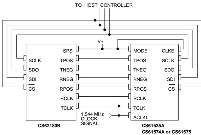
**Figure 3. Interfacing to a Crystal T1 LIU.**
