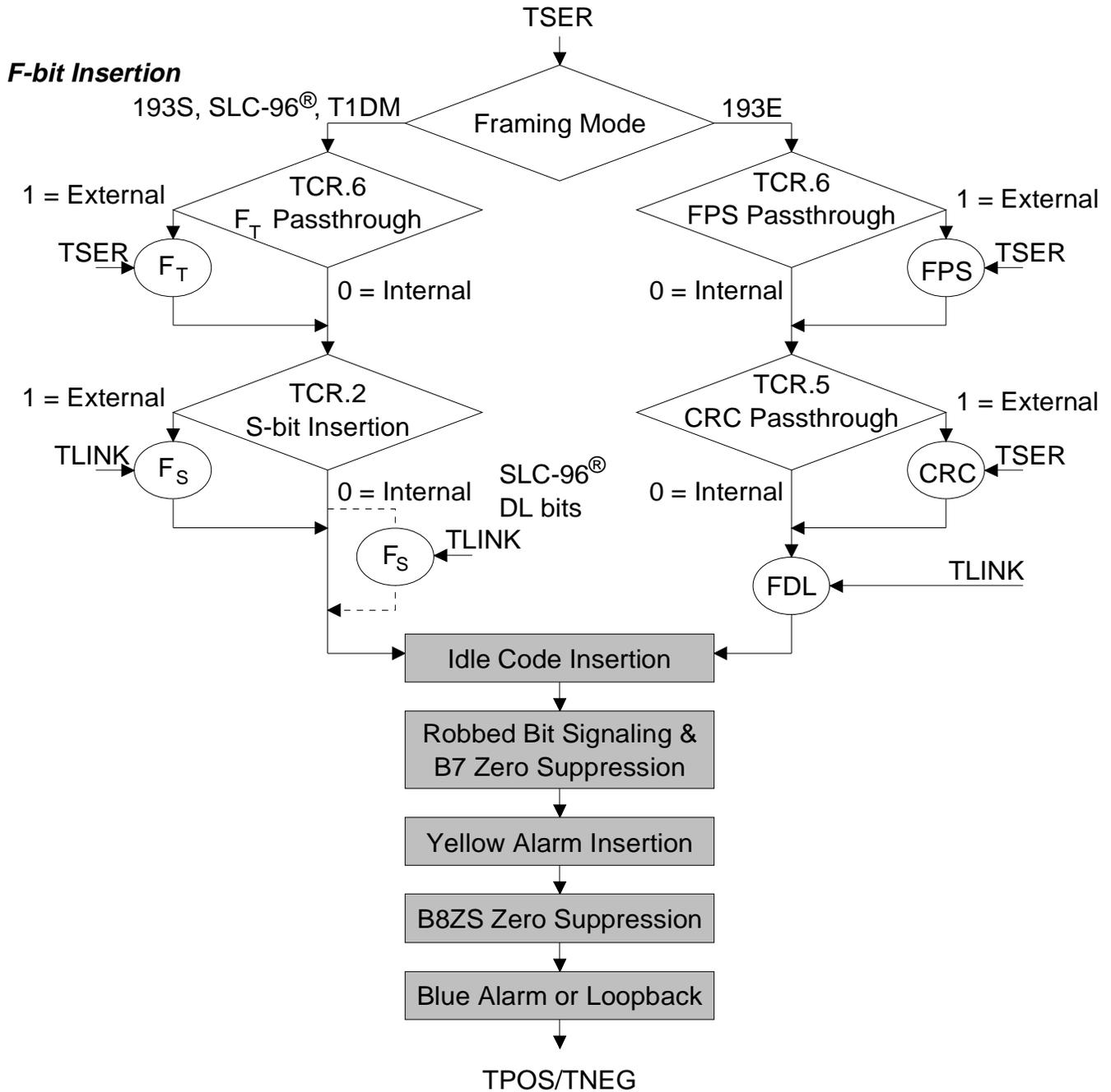
Figure 13a. Transmit Insertion Hierarchy: Framing Bits
