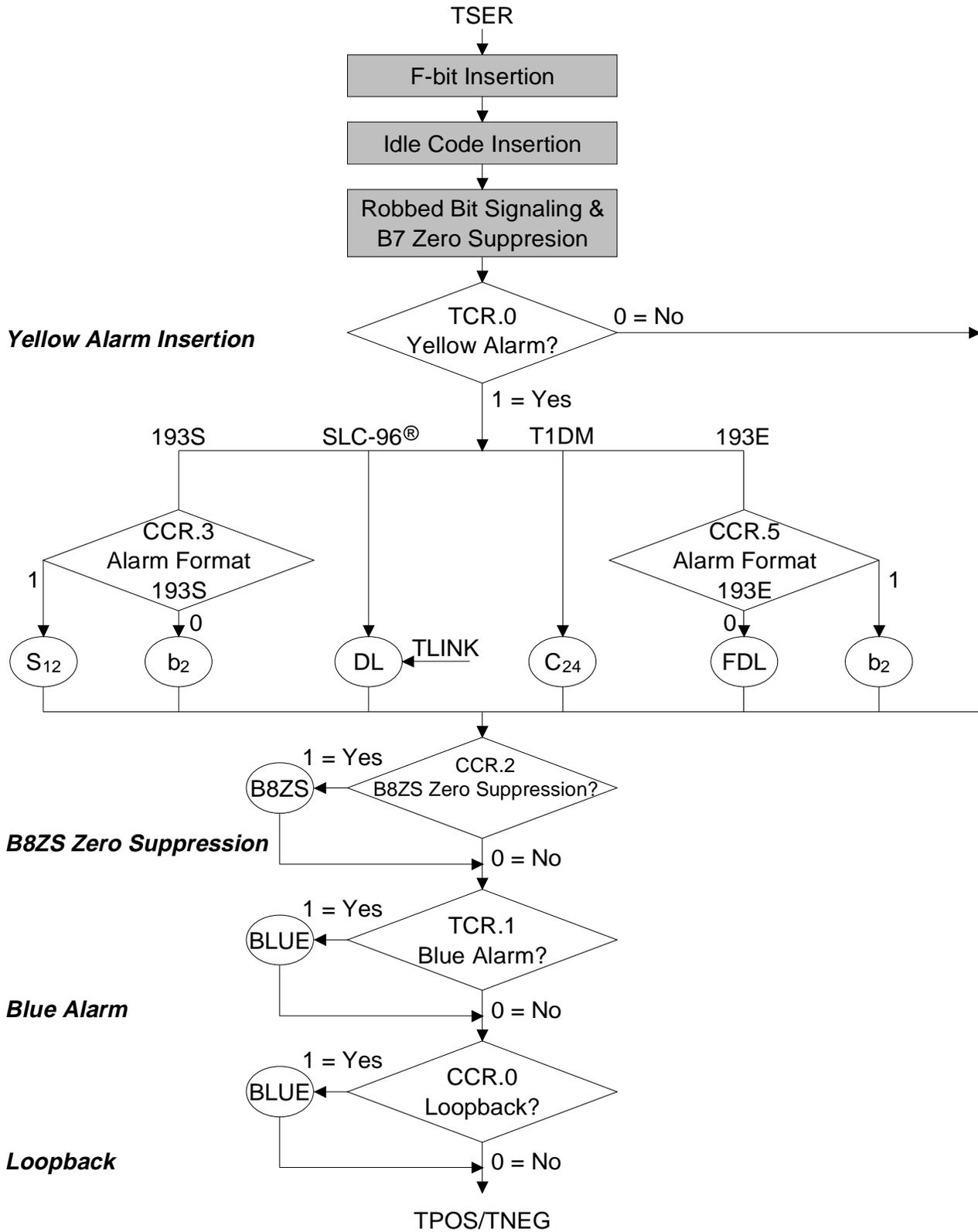
Figure 13c. Transmit Insertion Hierarchy: Alarms, B8ZS, and Loopback
