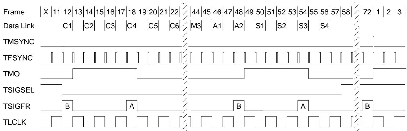
**Figure 8. SLC-96<sup>®</sup> Multiframing Transmit Timing**
