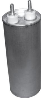
Type PC capacitors are designed to meet the demands of filter applications rich in system total harmonic distortion (THD). This series has a dual protection system utilizing self healing metallized polypropylene and a mechanical pressure interrupter to ensure a safe open circuit mode in the event of overload or end of life. (\*)
