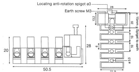
On CFTBN/1 spigot to mounting hole = 10mm
