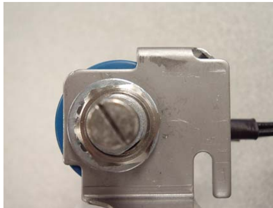
H-37-7 washer installed on bracket
