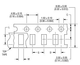
NOTES: TAPE MATERIAL IS PAPER. TAPE THICKNESS IS  $\frac{0.60\pm0.05}{(0.024\pm0.002)}$  COVER TAPE ADHESION IS 40  $\pm$  15 GRAMS.
