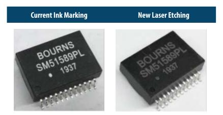
The laser etching process will have no impact on the fit or function of the product. The form will change due to the modification of the marking process to laser etching. The quality and reliability of the marking will be improved as the result of the process change. The following part numbers will be affected:
