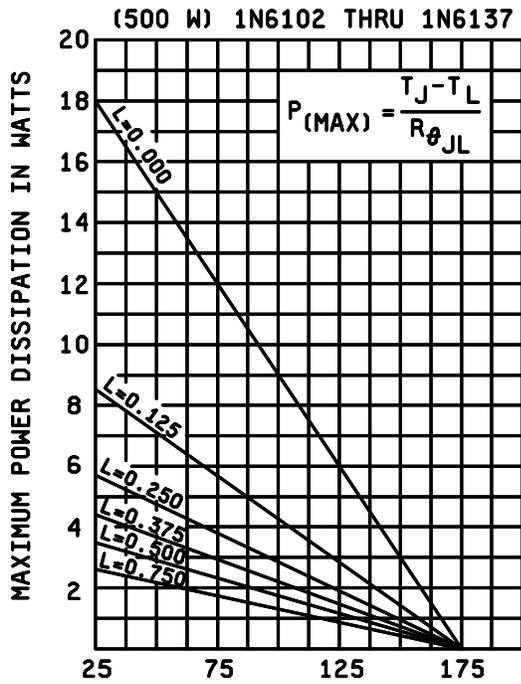
MAXIMUM LEAD TEMPERATURE IN °C ( $T_L$ ) AT POINT "L" FROM BODY (FOR MAXIMUM OPERATING JUNCTION TEMPERATURE WITH EQUAL TWO-LEAD CONDITIONS).
