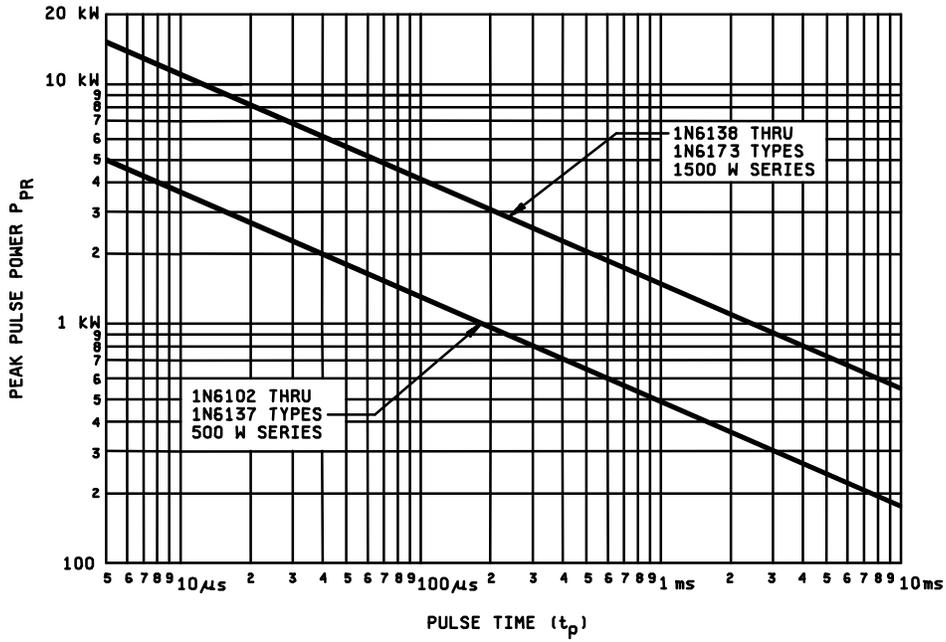
FIGURE 7. Peak pulse power versus pulse time.
