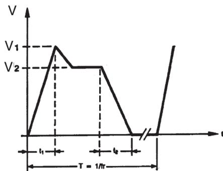
Choice of voltage:  $V_1 \leq V_{peak}$
