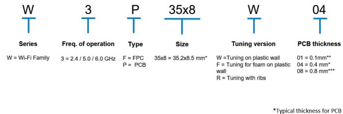
\* Thickness for PCB \*\* Thickness for FPC \*\*\*Recommended for assembly with ribs
