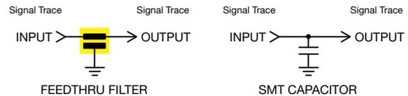
Figure 1. Comparison of Feedthru Capacitors to Discrete Capacitors
