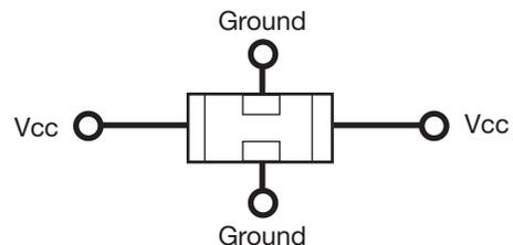
The terminals are connected internally side to side. Left side and right side are connected and front and back are connected internally.
