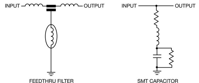
Figure 2. Comparison of Feedthru Capacitors to Discrete Capacitors
