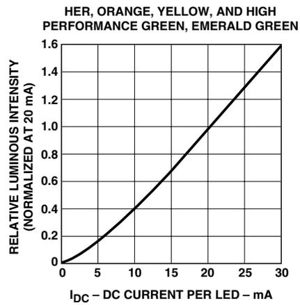
Figure 3. Relative luminous intensity vs. DC forward current.
