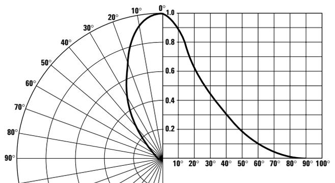
Figure 6. Relative luminous intensity vs. angular displacement for T-1<sup>3/4</sup> package.
