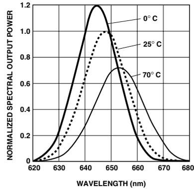
Figure 2. Typical spectra normalized to the 25°C peak.
