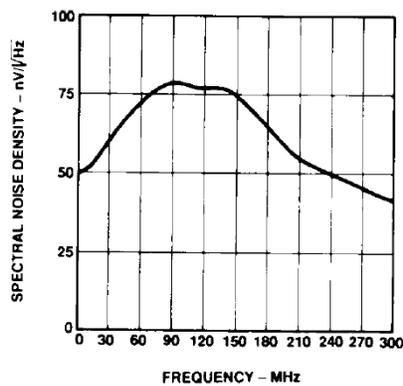
Figure 4. Typical output spectral noise density vs. frequency.
