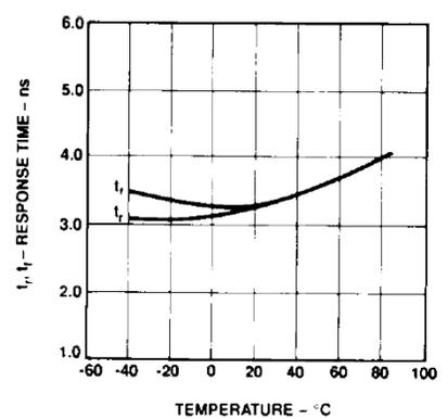
Figure 5. Typical rise and fall time vs. temperature.
