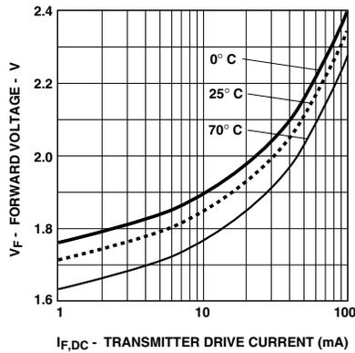
Figure 3. Typical forward voltage vs. drive current.
