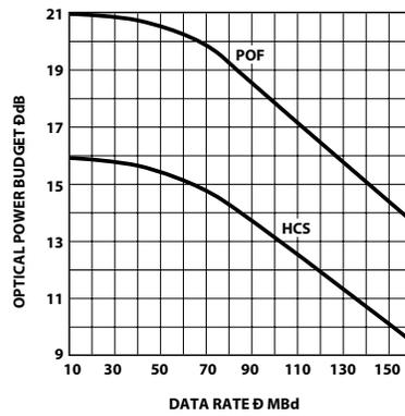
Figure 4. Typical optical power budget vs. data rate.
