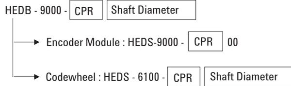
Note : The bundle part HEDB-9100/9000 consists of HEDS-9100/9000 and HEDS-5120/6100. The diagram below provides the breakdown list.
